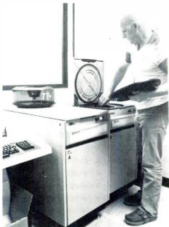
Figure 3. Senior editor Denis Mecham replaces the disk pack on one of the Century Data drive systems.
