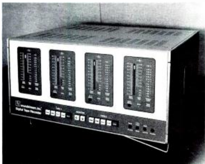
Figure 1. The Soundstream digital tape recorder's electronics emphasize data reliability first, with a minimum of bells-and-whistles on the front panel.
