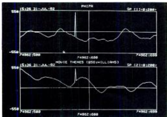
Figure 4. Expanded view of #3 with a scale of 200 samples or 1/250th of a second. Allows for either precise location of edit points or interpolation points for removal.
